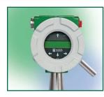
VorTek Instruments Pro-V<sup>™</sup> M24 Multivariable Vortex Flowmeter offers accurate and reliable flow metering in a multivariable design. The multivariable design incorporates a high-accuracy velocity sensor, a precision platinum RTD temperature sensor, and a solid-state pressure transducer. The M24 can deliver volumetric flow, mass flow, temperature, pressure, density, and energy (BTU) measurements
