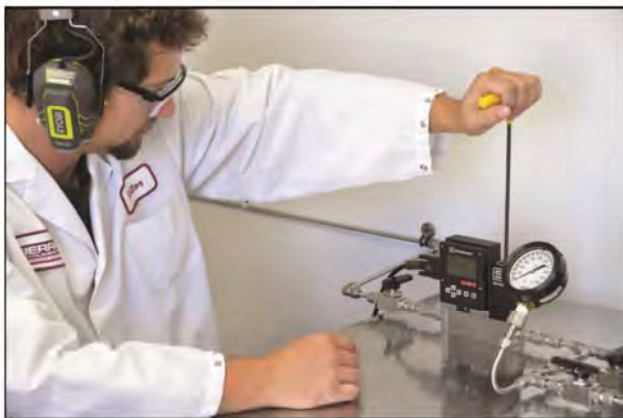
Mass Flow Controller Calibration: Valve Adjustment
