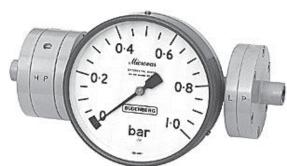
This instrument is generally used in applications where the system pressure is very much higher than differentialrange and can be used for measuring differential pressurein filters, strainers, coolers, pumps, natural gas strainers, orifice plates and venturi tubes.
