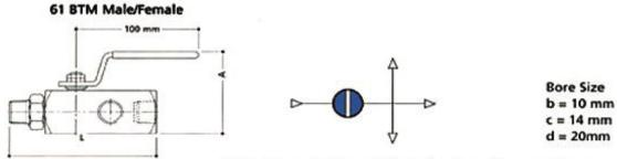
With one male inlet and three female outlet connections offers the facility with vent and blank plugs for localized venting.
